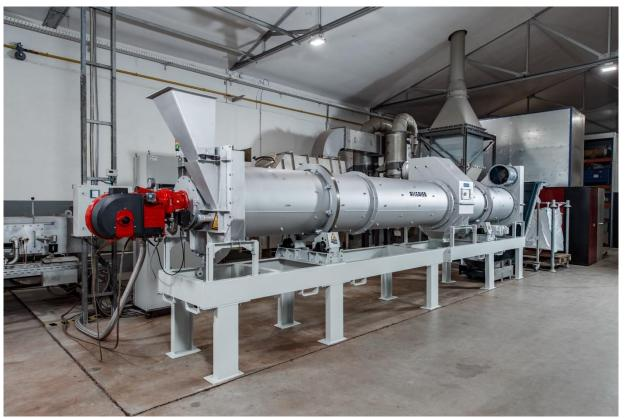
The new **TK-D** drum dryer / cooler system MOZER as a pilot plant in the Allgaier Test Center, Uhingen, Germany enables the solids to be dried to very low temperatures up to near ambient or cooling air temperatures
